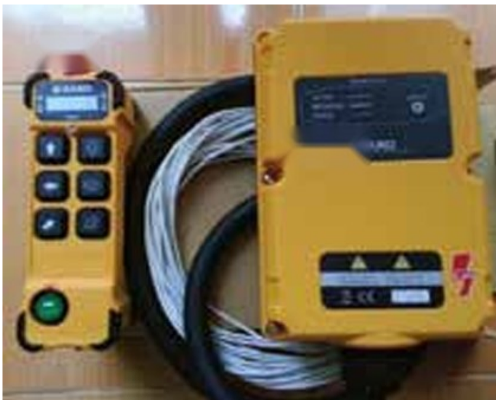
Radio remote control – Industrial radio control with emergency stop and receiver in the panel.
