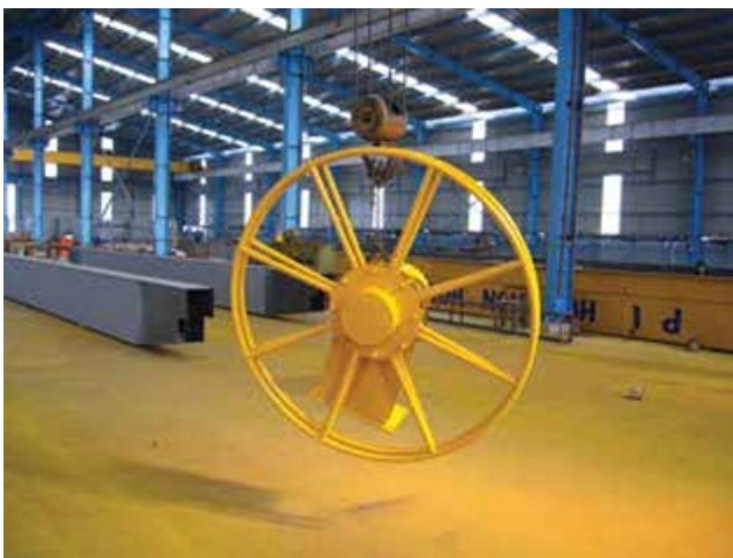
Cable reel – Spring or motor reel for power to mobile gantries and transfer carts.
